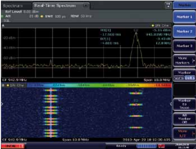
Spectrum and spectrogram of GSM signals on different frequency bands. Markers are used to measure a frame length of 4.6 ms.
